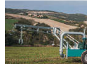
Bandiera porta aspirazione Arm-holder to lift up the suction pipe Bras pour soulever le tuyau d'aspiration
